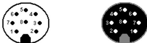
Figure 7: Pin code: Connection plug / socket for 8-pin version Connector cable pin configuration defined by manufacturer. The outlets may be re-programmed for specific applications.
